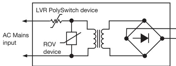
coupling the LVR device to the transformer can be accomplished either by making physical contact with the transformer or specifying that the transformer supplier design the LVR device into the transformer itself.
