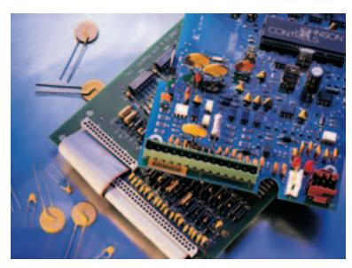
PolySwitch resettable devices can react to the faults that are caused by overcurrent and overtemperature conditions and can help to protect monitoring, sensing, and control systems.
