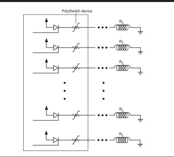
A protection scheme is also noted in Figure 4. Since these sensor lines can cover long distances, they are typically found in the same conduit with other voltages. If an overvoltage situation should occur, and the rail voltage of the op-amp is exceeded, the overvoltage device will immediately break down. The PolySwitch device will then trip if the fault is prolonged, helping to protect the circuitry, including the overvoltage device.
